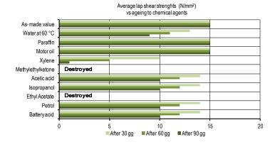
If not otherwise specified, the tests have been carried out at 20  $^{\circ}$ C after immersion for 30, 60 and 90 days at 20  $^{\circ}$ C on steel to steel joints which have been hardened for 48 hours at 20  $^{\circ}$ C.
