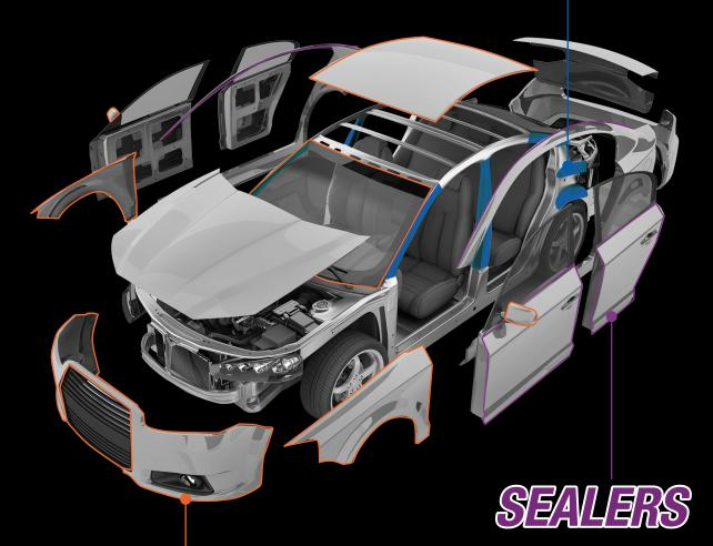
2k PU sealers are one of the most largely used products in the collision repair market. They keep out moisture and perfectly replicate the sprayed or brushed effect around door seals.
