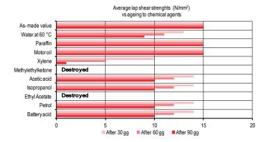
If not otherwise specified, the tests have been carried out at 20  $^\circ\text{C}$  after immersion for 30, 60 and 90 days at 20  $^\circ\text{C}$  on steel to steel joints which have been hardened for 48 hours at 20  $^\circ\text{C}.$
