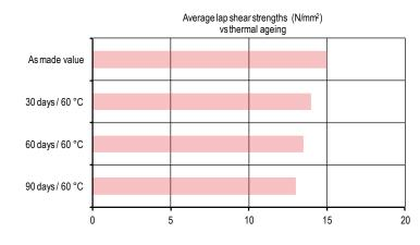
The tests have been carried out at 20 °C on steel to steel joints, which have been aged at 60 °C.
