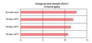
The tests have been carried out at 20 °C on steel to steel joints, which have been aged at 60 °C.
