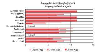
If not otherwise specified, the tests have been carried out at 20 °C after immersion for 30, 60 and 90 days at 20 °C on steel to steel joints which have been hardened for 48 hours at 20 °C.
